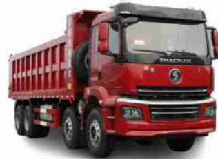
Brand: SHACMAN Model: E3 Engine: Cummins/Weichai 380-420HP Payload: 30-50 Ton Cargo box capacity: 20-30 m 3
