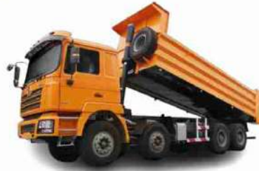
Brand: SHACMAN Model: F3000 Engine: Weichai 380-460HP Payload: 30-50 Ton Cargo box capacity: 20-30 m 3
