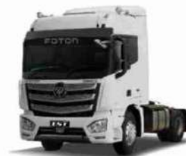
Brand: FOTON Model: EST Engine: Cummins 340HP-480HP Pulling Capacity:30-80 Ton Dimension:6105*2490*3570 mm
