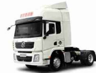
Brand: SHACMAN Model: X3000 Engine: Cummins 340HP-480HP Pulling Capacity: 30-80 Ton Dimension:6150*2550*3980 mm
