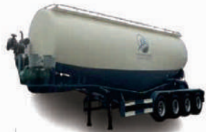
Bulk cement semi-trailer
