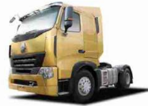
Brand: SINOTRUK Model: Howo A7 Engine: Weichai 336HP-480HP Pulling Capacity: 30-80 Ton Dimension:6260*2496*3850 mm
