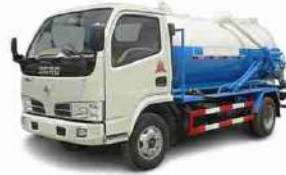
Sewage suction truck
