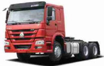
Brand: SINOTRUK Model: Howo HW76 Cabin Engine: Weichai 336HP-430HP Pulling Capacity: 40-100 Ton Dimension:6800*2496*2958 mm
