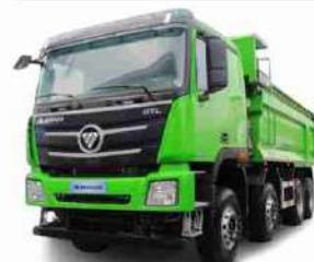
Brand: FOTON Model: ETX Engine: Cummins/Weichai 300-430HP Payload: 30-50 Ton Cargo box capacity: 20-30 m 3
