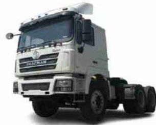
Brand: SHACMAN Model: F3000 Engine: Weichai 270HP-460HP Pulling Capacity: 40-100 Ton Dimension:6825*2490*3624 mm
