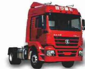
Brand: SHACMAN Model: M3000 Engine: Weichai 336HP-430HP Pulling Capacity: 30-80 Ton Dimension:5985*2490*3910 mm
